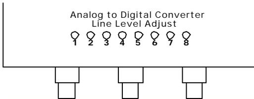
There is typically a 14dB difference between the 0dB reference levels in analog and digital equipment. The line level adjust on the FIREstation allows the user to adjust the 0dB reference to match that of an external analog device such as a preamp or console. A tweaker or small Phillips screwdriver can be used to adjust this level. Turn the tweaker clockwise to raise the 0dB level and counter-clockwise to lower the level.
