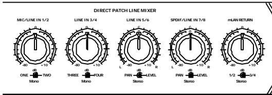
All 12 channels of the line mixer are routed directly to the Headphone/Main Output volume control knobs/outputs. Every two/four (according to the signal designation) channels are grouped together sequentially to one dual concentric knob.
