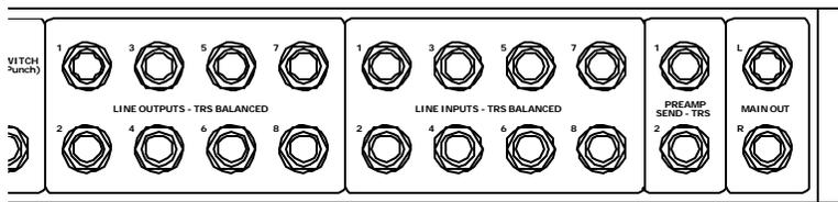
The TRS inputs and outputs are designed for use with balanced or unbalanced 1/4" cables. Balanced cables have an extra conductor and allow a signal to be sent over a longer distance while maintaining a lower noise floor. The TRS line inputs for channels one and two take precedent over preamp channels one and two. This is done so that another device may be placed between the preamp sends and the TRS line inputs.
