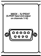
An external breakout cable is provided with the FIREstation to provide MIDI I/O and S/PDIF I/O. The S/PDIF I/O accepts a coaxial plug and does not accept an optical plug without a converter (coaxial to optical and vice-versa).
