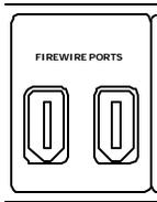
The IEEE1394 ports are 6-pin connectors. Both ports are bi-directional. They send and receive data from the other interconnected devices. IEEE 1394 compatible devices such as keyboards, computers, camcorders, etc. may be connected to the FIREstation using these ports.
