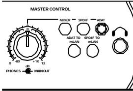
Another stand-alone mode occurs when just the ADAT button is pressed. In this mode, the FIREstation acts as an ADAT line mixer or converter. The ADAT signal can be converted to analog while being routed through the line mixer. It is important to note that the analog inputs are not functional in this mode.
