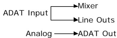
*NOTE: When using the FIREstation as an Analog to Digital (A-D) converter, the line mixer does not contain the analog inputs, just the ADAT inputs.*
