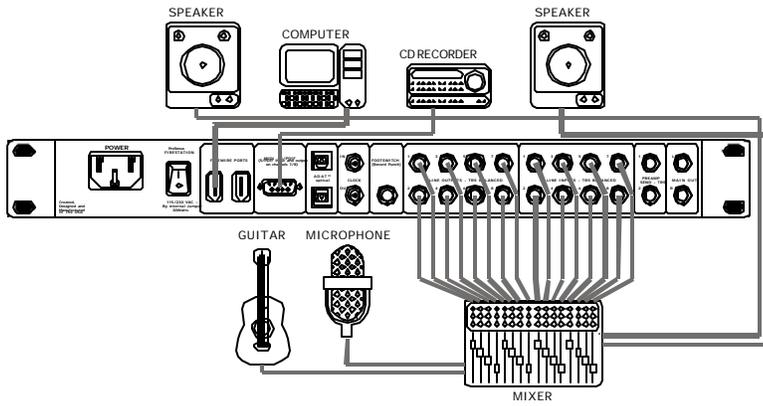
External mode incorporates other equipment beyond the FIREstation. For example, an external mixer and other processors may be used. In this mode, the outputs of the FIREstation could be routed to external equipment for dynamics processing, effects and other forms of manipulation. The master outputs could then be returned to two channels of the FIREstation to record the "Master Mix".
