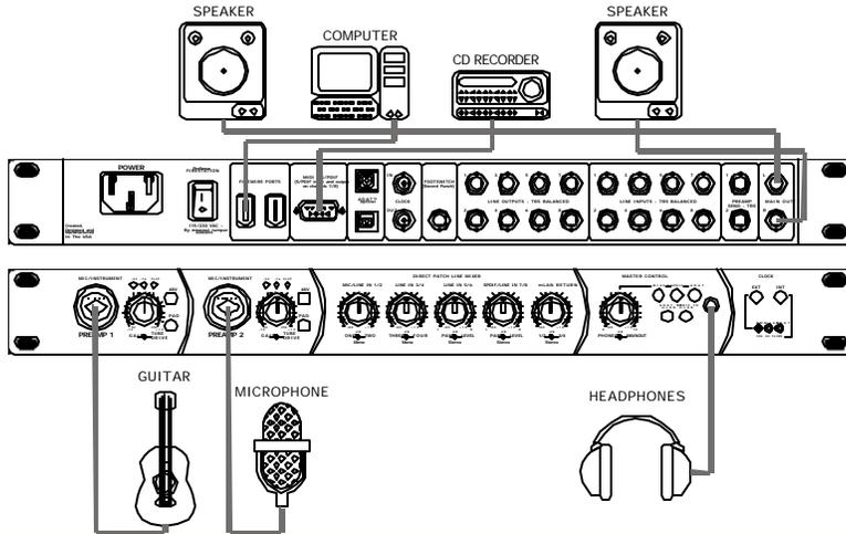
Internal mode signifies that you are using software and internal plug-ins to mix a project. In this instance only the master outputs and headphone outputs would be used. The internal mode is preferred in some situations dependent on the environment and other factors. For example, wouldn't it be nice to mix a song over headphones while sitting in a hotel room between live performances?
