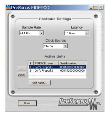
The control panel includes drop down menus to select samplerate, latency, and clock source, as well as an Active Units Panel
