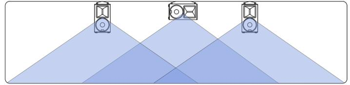
In contrast, the Pivot X110 horn achieves wide (110°), consistent horizontal coverage, while narrowly focusing the coverage in the vertical (50°) so that the high-frequency content has a longer throw. The resulting pattern expands with constant spectral content throughout the coverage area and all the way to its edges.
