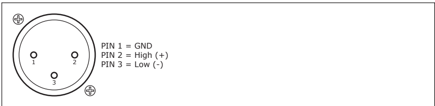
Cable Wiring Diagram for Input and Output XLR
