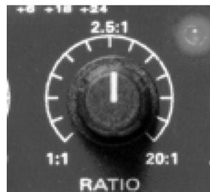
Ratio sets the compression slope. This is defined as the output level versus the input level. For example, if you have the ratio set to 2:1, any signal levels above the threshold (note: threshold is a preset parameter in the Blue Max) will be compressed at a compression ration
