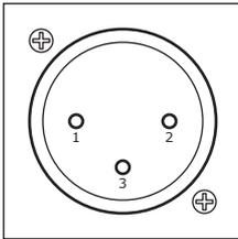
A switch labeled +48V is located next to each gain knob. This switch may be engaged to provide phantom power for condenser mics and any other device which may require phantom power by way of the XLR input. This power is supplied at a constant rate to allow use of all eight inputs simultaneously, without any degradation of audio quality. *Pin 1 = GND, Pin 2 = +48V, Pin 3 = +48V*
