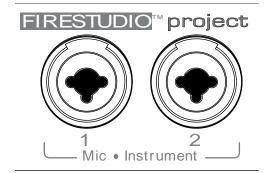
• <u>Instrument Inputs (Channels 1 and 2).</u> The ¼" TS connector on Channels 1 and 2 are for use with an instrument (guitar, bass, etc.). When an instrument is plugged into the ¼" input, a high impedance input buffer is switched into the preamp circuit and the FireStudio Project becomes an active instrument preamplifier.
