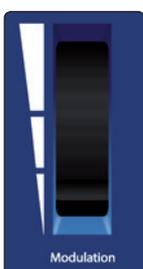
**Modulation Wheel.** By default, the modulation wheel is assigned to MIDI Continuous Controller 01, Modulation. This controller is often used to control a vibrato effect but the instrument preset you are controlling will determine what exactly is being modulated.
