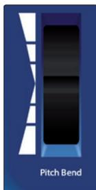
**Pitch-Bend Wheel.** The pitch-bend wheel is used to bend the notes up or down. How far you can bend a note up or down is determined by the MIDI instrument preset you are controlling. For example, if you are controlling a violin sample that only allows you to bend a note one half step, moving the pitch-bend wheel all the way up will only result in a half-step change.
