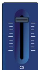
**Volume Slider.** By default, the volume slider is assigned to MIDI Continuous Controller 07, Channel Volume. It sends values from 0 to 127.
