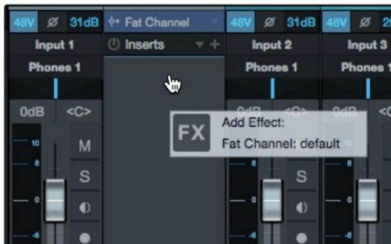
By default, the “link to DSP” button will be enabled. This links the parameters between the Mixer Fat Channel and the Fat Channel plug-in in Studio One. Editing either will change both.
