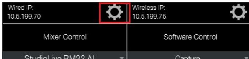
*NOTE: Connecting the CS18's Wireless interface is done in a similar fashion. With the Wifi adapter inserted, press the Gear icon for the Wireless interface, then press the **Network:** button to select your desired Wifi network*
