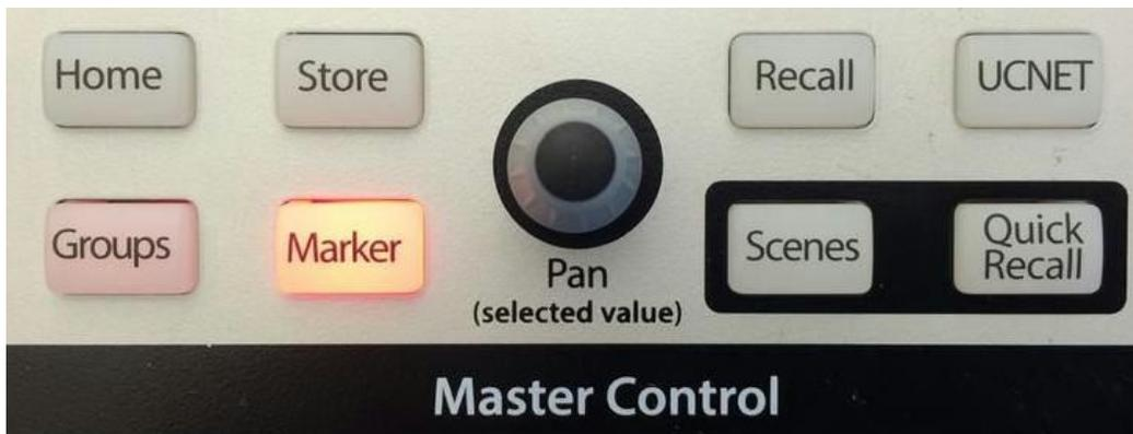
This screen allows navigation for jumping to individual markers, and markers can be added or removed. Also, the Pan encoder can be used as a jog wheel when the “Jog” button is selected on the LCD.
