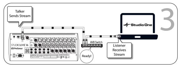
AVB streams are only forwarded once a successful reservation is made. After the streams stop, switch resources are then released and the process can begin again or make room for other network traffic. In this way, the AVB standard ensures that audio data streams always have the highest QoS and all other data is secondary or tertiary.
