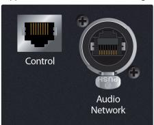
For StudioLive Series III mixers, the Audio Network connection should attach to the AVB network, while the control port should be connected to a wireless router, or an access point, so that the mixer can be controlled remotely from UC Surface or QMix-UC.
