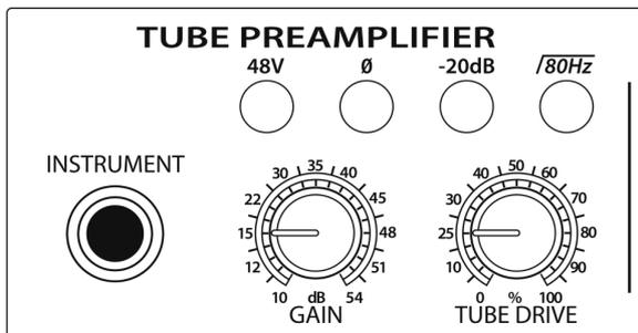
**Instrument Input.** The ¼" TS connector on the front panel is for use with a passive instrument (guitar, bass, etc.). When an instrument is plugged into the instrument input, the microphone preamp is bypassed, and the Studio Channel becomes an active instrument preamplifier.
