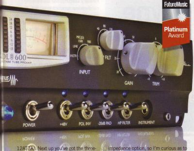
position high-pass filter (40Hz, 80Hz and 120Hz @ 6dB per octave) and then the 'trim' circuit. This uses the second 6922 valve, offering 10dB continuously variable cut and boost.
